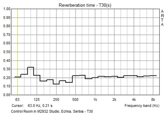
Figure 7 T30 results in first Control Room done by new principles
