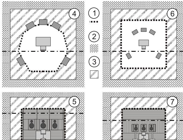
Fig. 1. – Some possible ways of MyRoom design: 1. air-transparent diffuse surface, 2. stiff wall, 3. low frequency absorption, 4. horizontal cross-section of room with soffit monitors, 5. vertical c.s. of room with soffit monitors, 6. horizontal c.s. of room with free-standing monitors, 7. vertical c.s. of room with free-standing monitors.
