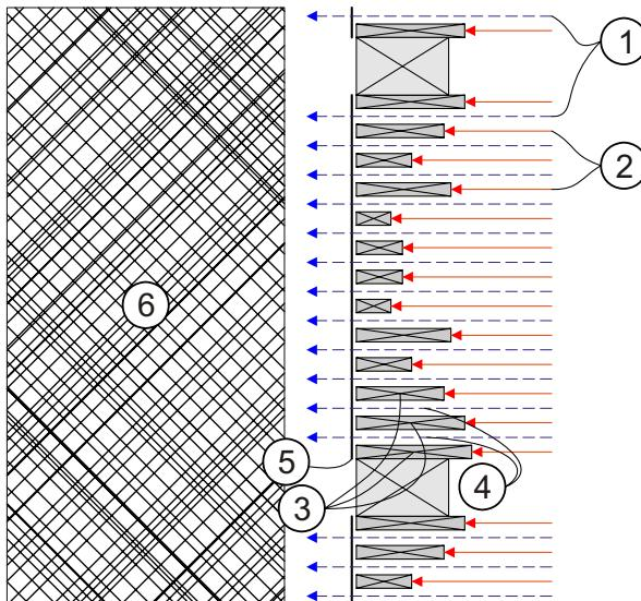
Fig. 2. – Side wall applied MyRoom treatment principle, horizontal cross-section, (top view): 1. air waves which pass through (blue/absorbed/diffused), 2. Air waves which cannot pass through (red/reflected/diffused), 3. Diffuser slats, 4. “Through hole” wells, 5. air transparent fabric, 6. Wideband absorber.
