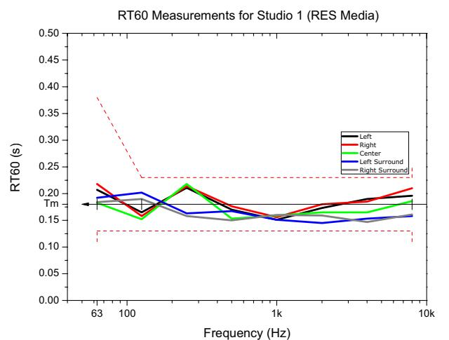
Fig. 3. - RT60 Frequency dependence for the control room in the RES Media Studio, with AES limitations [9].
