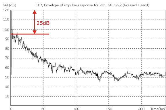
Fig. 7. – Pressed Lizard Control Room with stereo monitoring. Envelope of impulse response.
