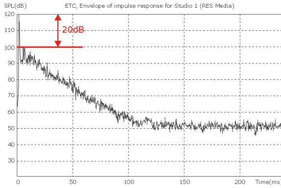
Fig. 4. – Envelope of impulse response for RES Media Studio. Similarities with Blackbird Studio C are obvious, only attenuation of first reflections isn't 30dB.
