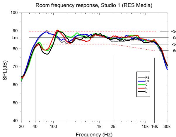
Fig. 5. – Acoustical frequency response of the surround control room in the RES Media Studio along with the limits defined in AES recommendations [9]. Graph shows the response of all five speakers.
